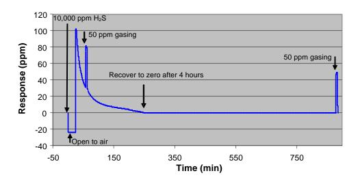
Figure 2. Response and Recovery of Electrochemical Sensor from Exposure to 10,000 ppm H₂S.
