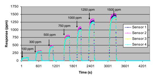
Figure 1. Response of Solid State Sensor after Calibration with 100 ppm H<sub>2</sub>S.
