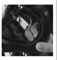
4. Rotate the spectacles horizontally by sliding prongs in the rubber block.
